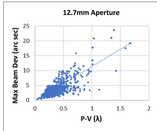
Figure 6. Chart showing that on smaller parts with smaller beam deviations, retroreflectors can depart from theoretical linearity
