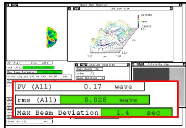
In the double-pass set up the PV values are very close, yet the resulting beam deviation is different by nearly a factor of two.
