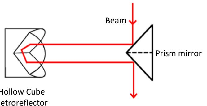
Figure 5. Optical Delay Line
