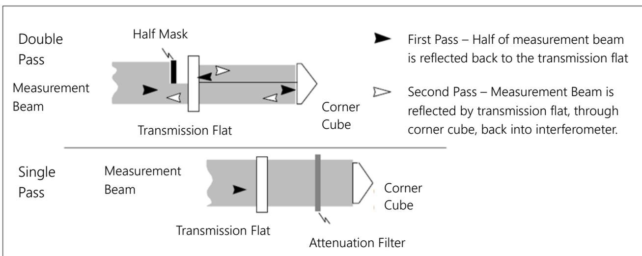
Figure 7. Fizeau Interferometer Layout. Image courtesy of Zygo® Corporation
