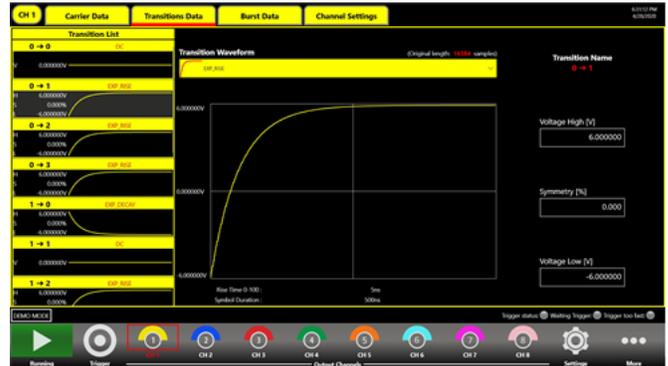
The software architecture provides the possibility to easily generate the patterns in different generation modalities and also gives the opportunity to modulate the patterns with internal or external signals with the purpose to generate also different effects of noise (jitter, ripple, ...).
