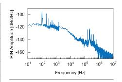
Signal at 1.7 µm: RMS 0.15 %
