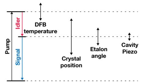
TOPO tuning mechanisms (Figure 1b)
